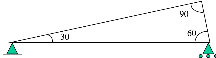
hinge: transmits both vertical and horizontal forces at the surface
