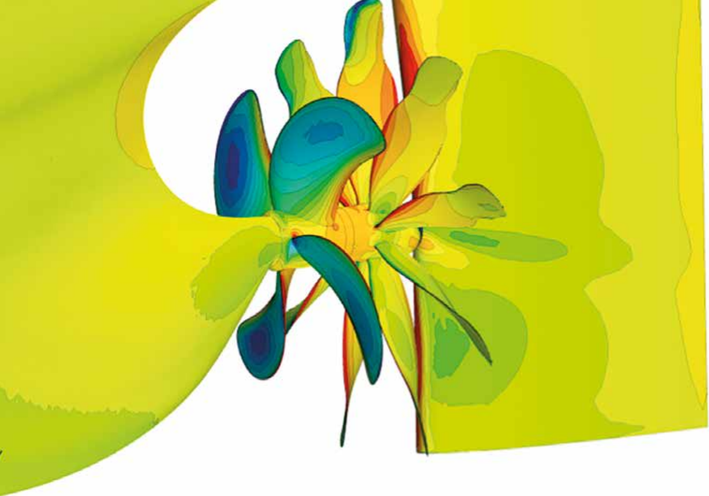
Figure 2: Model of a complete propulsion system in Simcenter STAR-CCM+.
