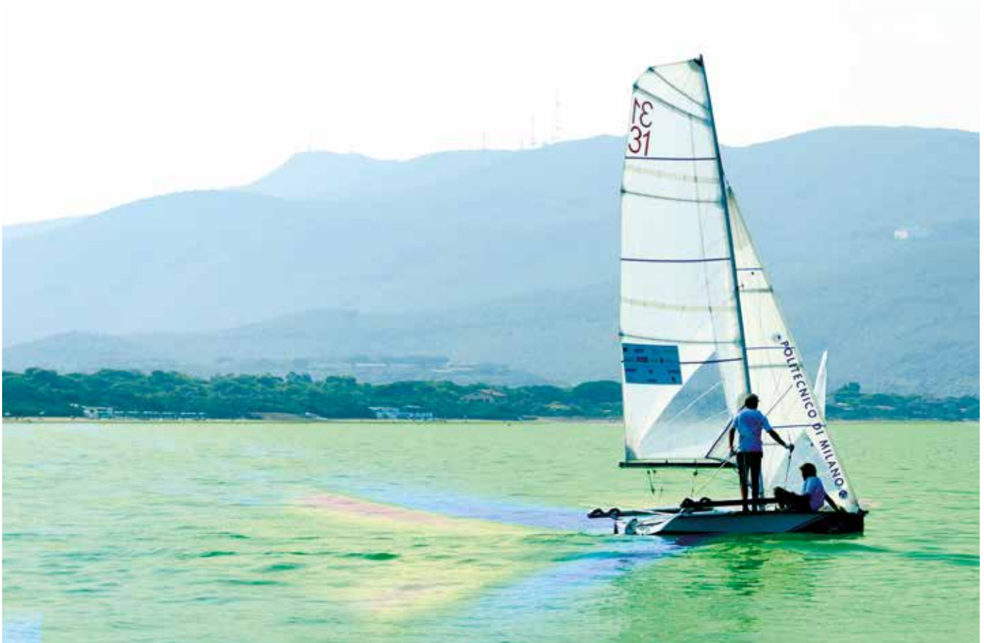
Figure 1: A photograph of the R3 skiff sailing upwind and the overlaid results of the hydrodynamic simulations.
