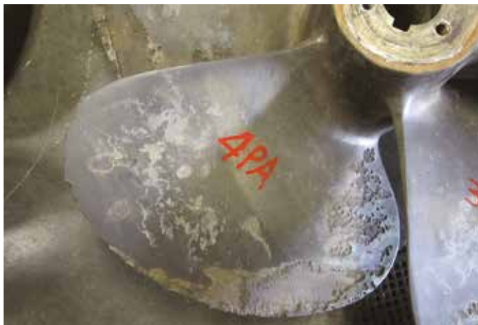
Propeller with cavitation damage.
