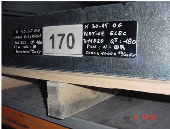
Fig. 8.44 Supermarket of unpainted sheet metal parts
