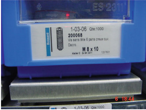
Fig. 8.47 Containers on electrical scale
