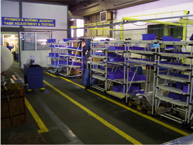
Fig. 8.85 Tanks in one piece flow line – supply side
