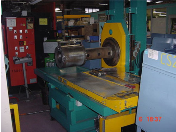
Fig. 8.37 Coils bending machine at the final assembly line
