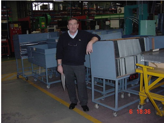
Fig. 8.41 Supermarket for sheet metal parts
