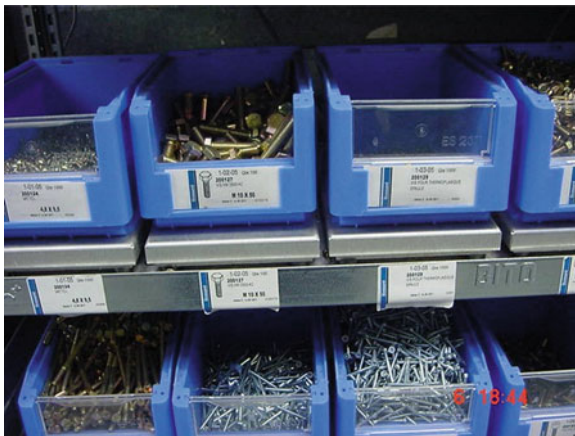
Fig. 8.46 Supermarket for small parts – in detail
