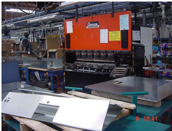
Fig. 8.36 Brake press at the assembly line
