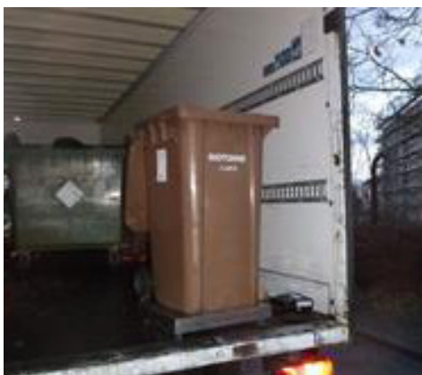
F-01: Sampling of smaller bins, compiling to a 1.1 m3 container, with mobile weighbridge
