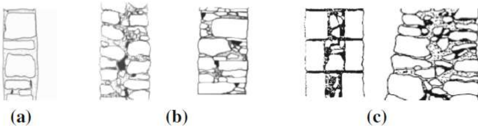
Fig. 2 Classification of masonry in respect to wall sections (morphology) (Binda and Cardani 2007). a Single leaf, b double-leaf, c three-leaf
