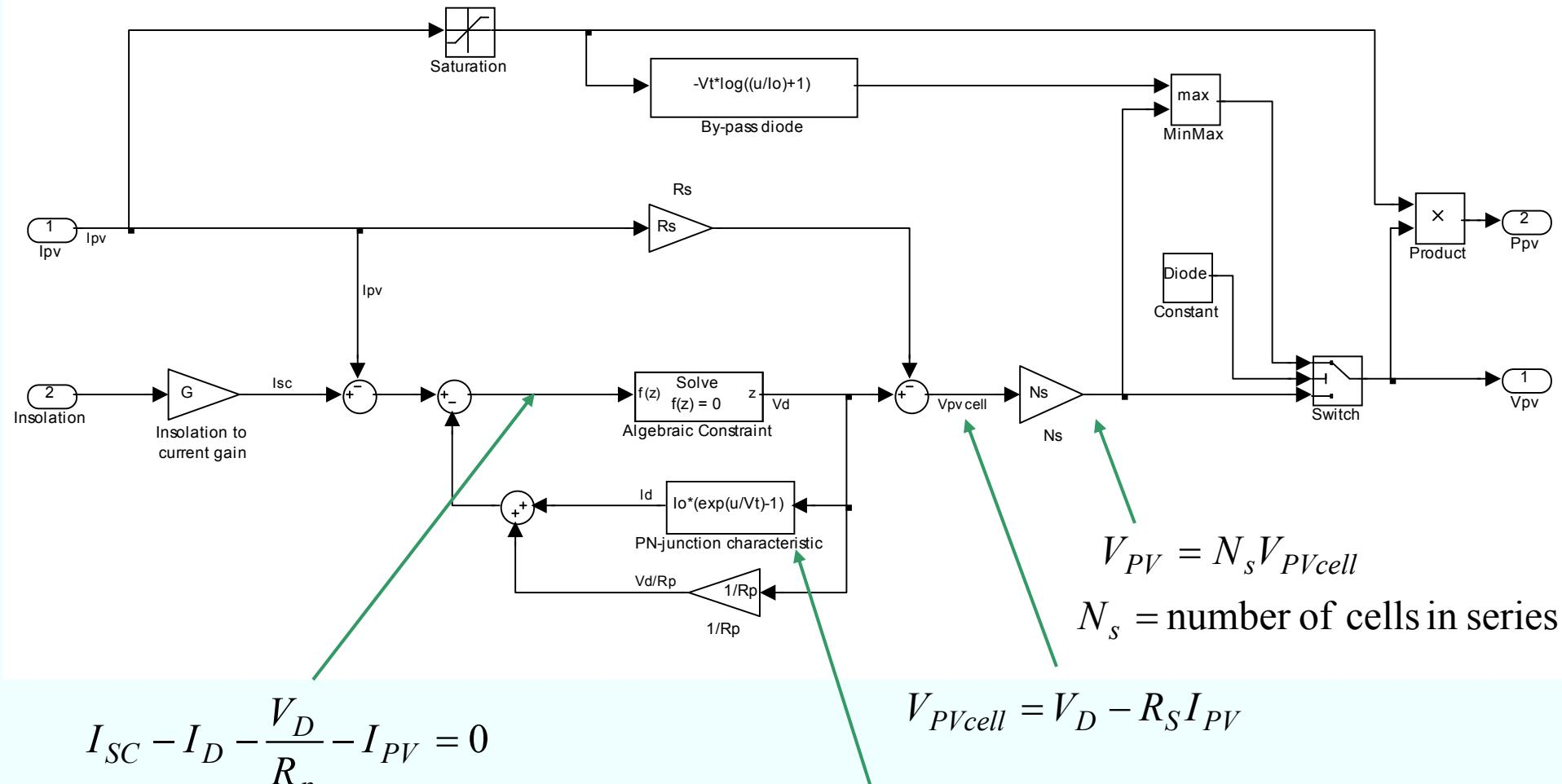
$$I_{SC} - I_D - \frac{V_D}{R_p} - I_{PV} = 0$$
