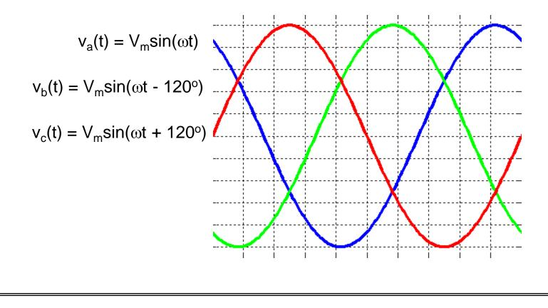
$$\overline{v} = \frac{2}{3} \left( v_{a}(t) + a v_{b}(t) + a^{2} v_{c}(t) \right)$$
