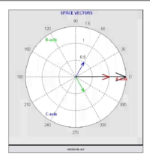
Three phase quantities vary sinusoidally with time (frequency f)
