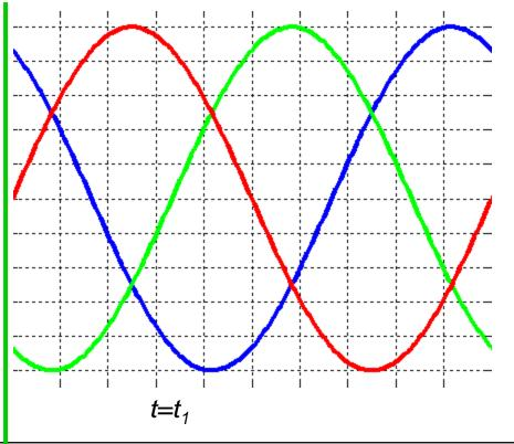
$$\overline{v} = \frac{2}{3} \left( v_{a}(t) + a v_{b}(t) + a^{2} v_{c}(t) \right)$$
