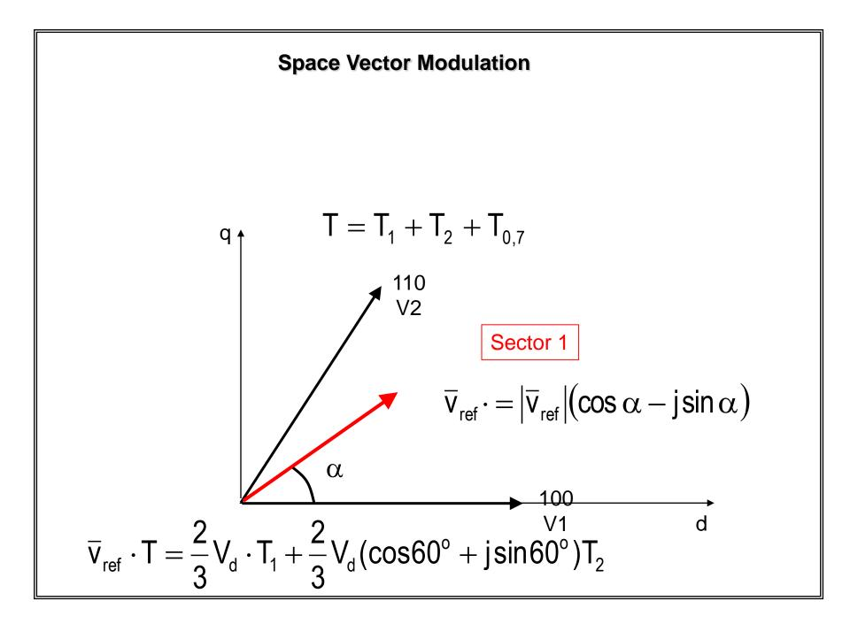
$$\overline{V}_{ref} \cdot T = \frac{2}{3} V_d \cdot T_1 + \frac{2}{3} V_d (\cos 60^\circ + j \sin 60^\circ) T_2$$
