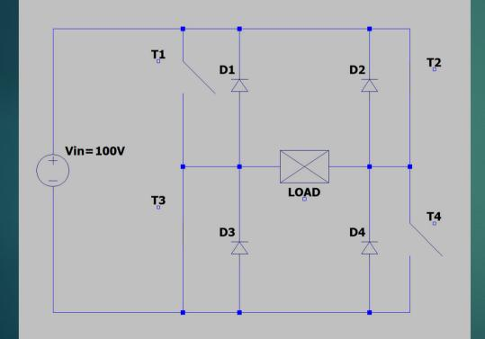
When transistors T2, T3 are pulsed, the voltage on load is V0 = -100V
