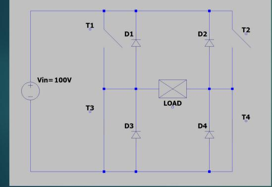
When the transistors T3, T4 are pulsed, the voltage on load is V0 = 0V, regardless of the load current flow.
