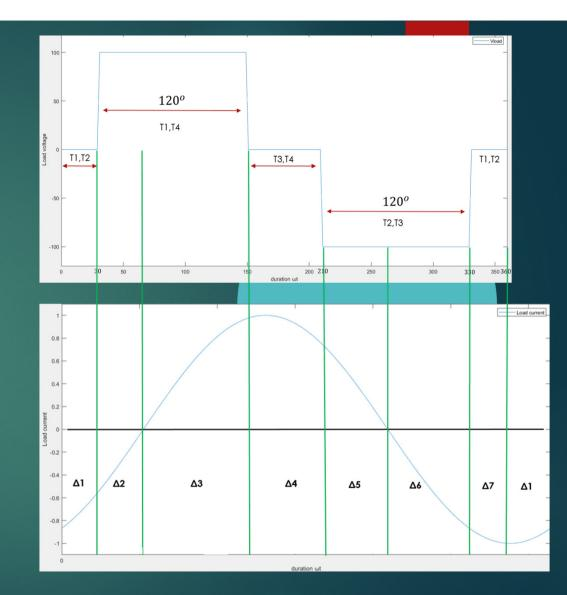
Positive voltage and negative current -> negative power(V0 \* I0 < 0), energy is transferred from load to source. In conduction: D1,D4.
