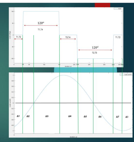
Positive voltage and positive current-> positive power (V0 \* I0 > 0), energy is transferred from source to load. In conduction : T1,T4.
