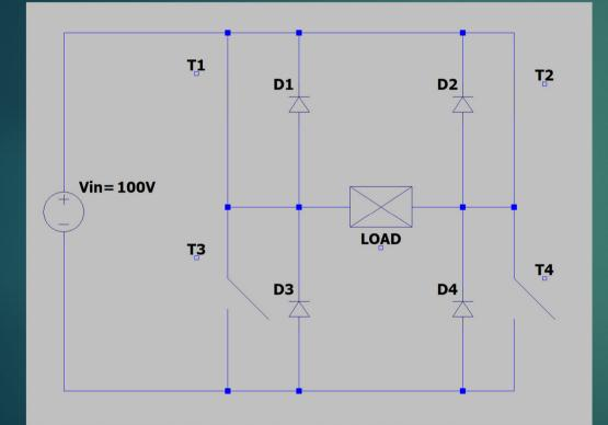
When transistors T1, T2 are pulsed, the voltage on load is V0 = 0 V, regardless of the current flow.
