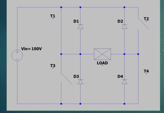
When transistors T1, T4 are pulsed, the voltage on load is V0 = 100V
