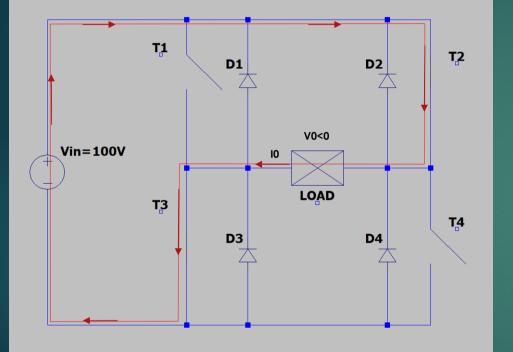
Negative voltage and negative output current -> positive power (V0 \* I0 > 0), energy is transferred from source to load. In conduction : T2,T3.
