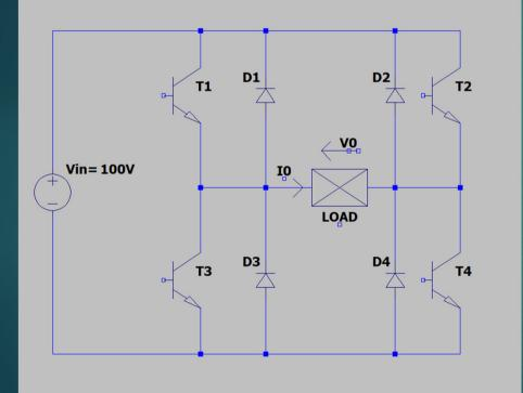
For the inverter of the adjacent figure, design the ignition pulses of the transistors, so that the output voltage of the inverter consists of rectangular pulses of 120° width
