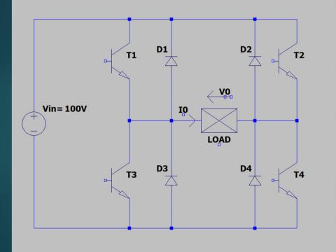
For the inverter of the previous example, the voltage and current waveform are shown above. What are the waveforms of current of the semiconductor devices?
