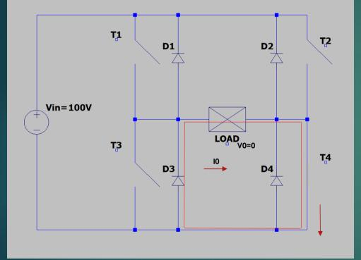
0 voltage and positive output current -> zero power (V0 \* I0 = 0), there is no energy transfer. In conduction : T4,D3.
