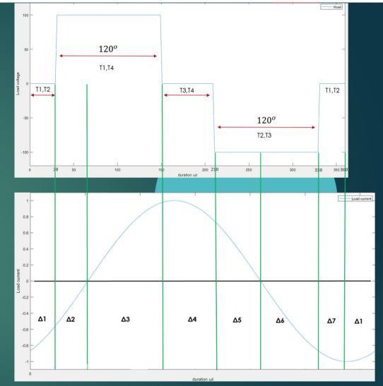
0 voltage and negative output current -> zero power (V0 \* 10 = 0), there is no energy transfer. In conduction: D1,T2
