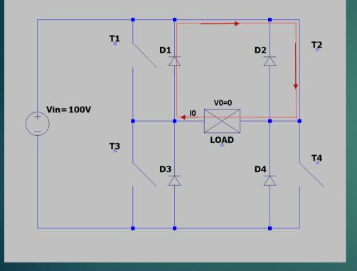
0 voltage and negative output current-> zero power (V0 \* I0 = 0), there is no energy transfer. In conduction : D1,T2.
