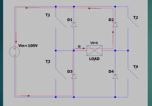
Negative voltage and positive output current-> negative power (V0 \* I0 < 0), energy transferred from load to source. In conduction : D2,D3.
