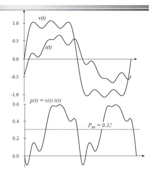
Root-mean-square (RMS) value of a waveform, in terms of Fourier series
