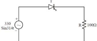
The circuit is that of a single phase half wave controlled rectifier with a resistive load
