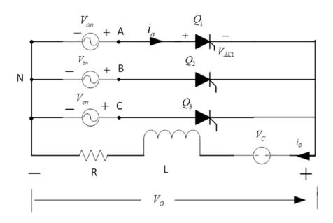
If any one supply line is disconnected, the circuit behaves like a single phase half controlled rectifies with RL load.
