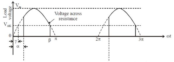
It is observed that the SCR turns off when  $\omega t = \beta$ , where  $\beta = (\pi - \gamma)$  because the SCR turns-off for anode supply voltage below 1 Volt.
