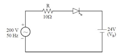
It is obvious that the SCR cannot conduct when the instantaneous value of the supply voltage is less than 24 V, the battery voltage. The load voltage waveform is as shown (voltage across ion).
