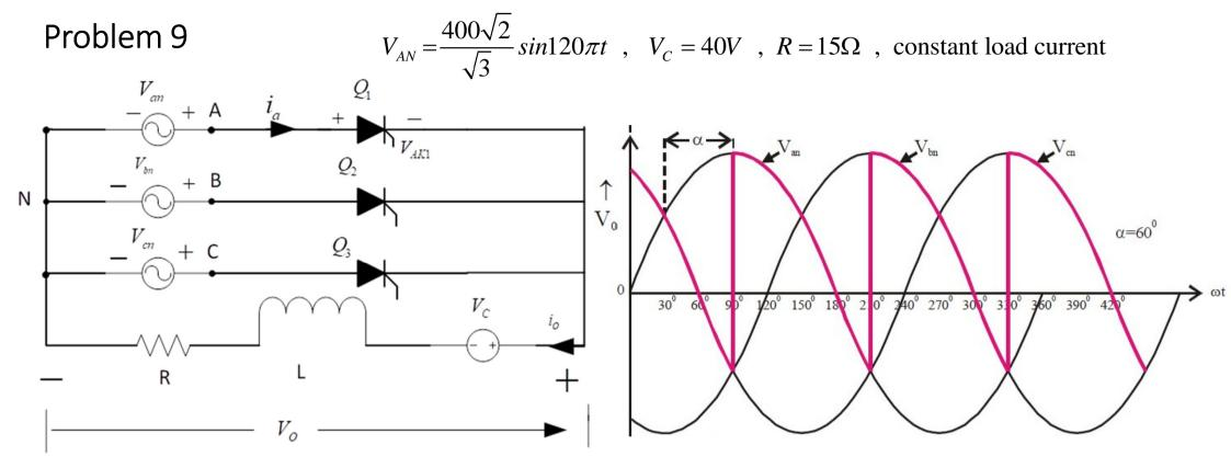
Calculate average and RMS load current values,  $\alpha = 60^{\circ}$
