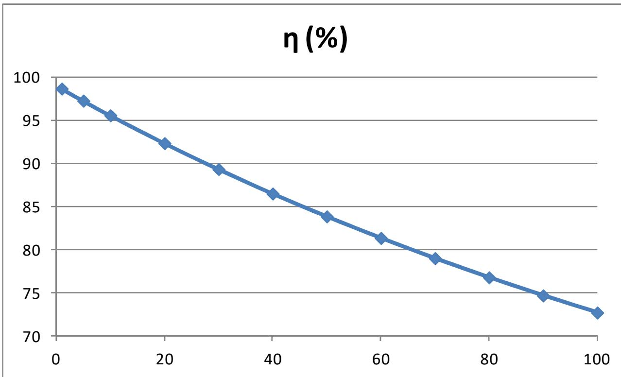
$$\begin{aligned}P_{loss}(W) &= P_{Cond} + W_{SW} f_s \Rightarrow \\ \Rightarrow P_{loss}(W) &= 20 + 7,3 \cdot f_s(kHz) \\ P_o(W) &= V_o I_o = 2000W \\ \eta(\%) &= \frac{P_o}{P_{in}} 100\% = \frac{P_o}{P_o + P_{loss}} 100\% = \\ &= \frac{1}{1 + \frac{P_{loss}}{P_o}} 100\% = \frac{1}{1 + \left[ \frac{(20 + 7,3 f_s)}{2000} \right]} 100\%\end{aligned}$$
