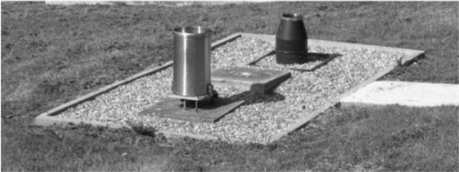
Tipping bucket rain gauge (foreground) and storage gauge (background) in southern England. Photo: Y. Chen (Copyright © Environment Agency 2009 all rights reserved)
