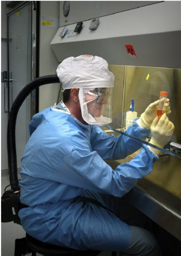
FIGURE 4.14 Biosafety facility. Researcher at US Centers for Disease Control working with the influenza virus under biosafety level 3 (BSL-3) conditions, with a respirator inside a biosafety cabinet.
