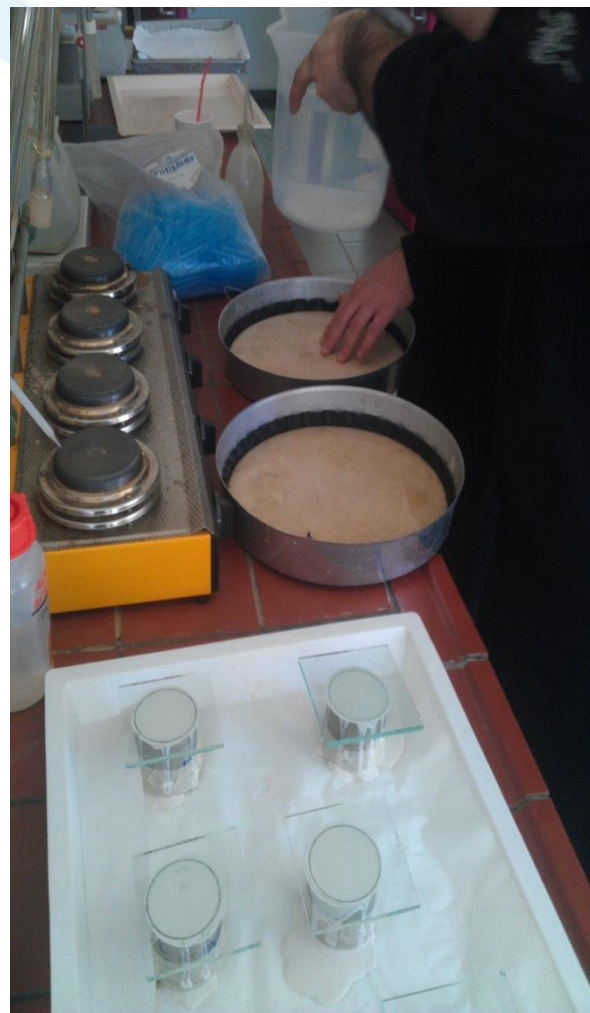
Pressure plates saturation process
