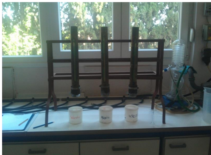
Array of devices for the determination of saturated hydraulic conductivity using the falling head method
