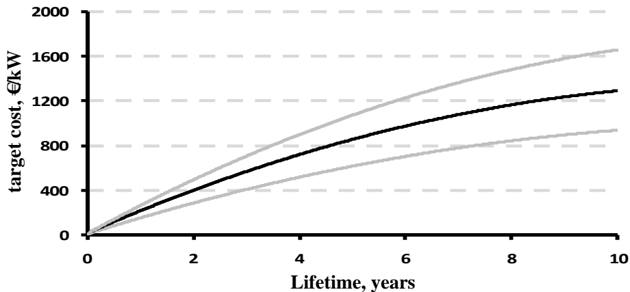
Figure 5 Estimated effect of fuel cell lifetime on the target cost for competitive commercialization [35]
