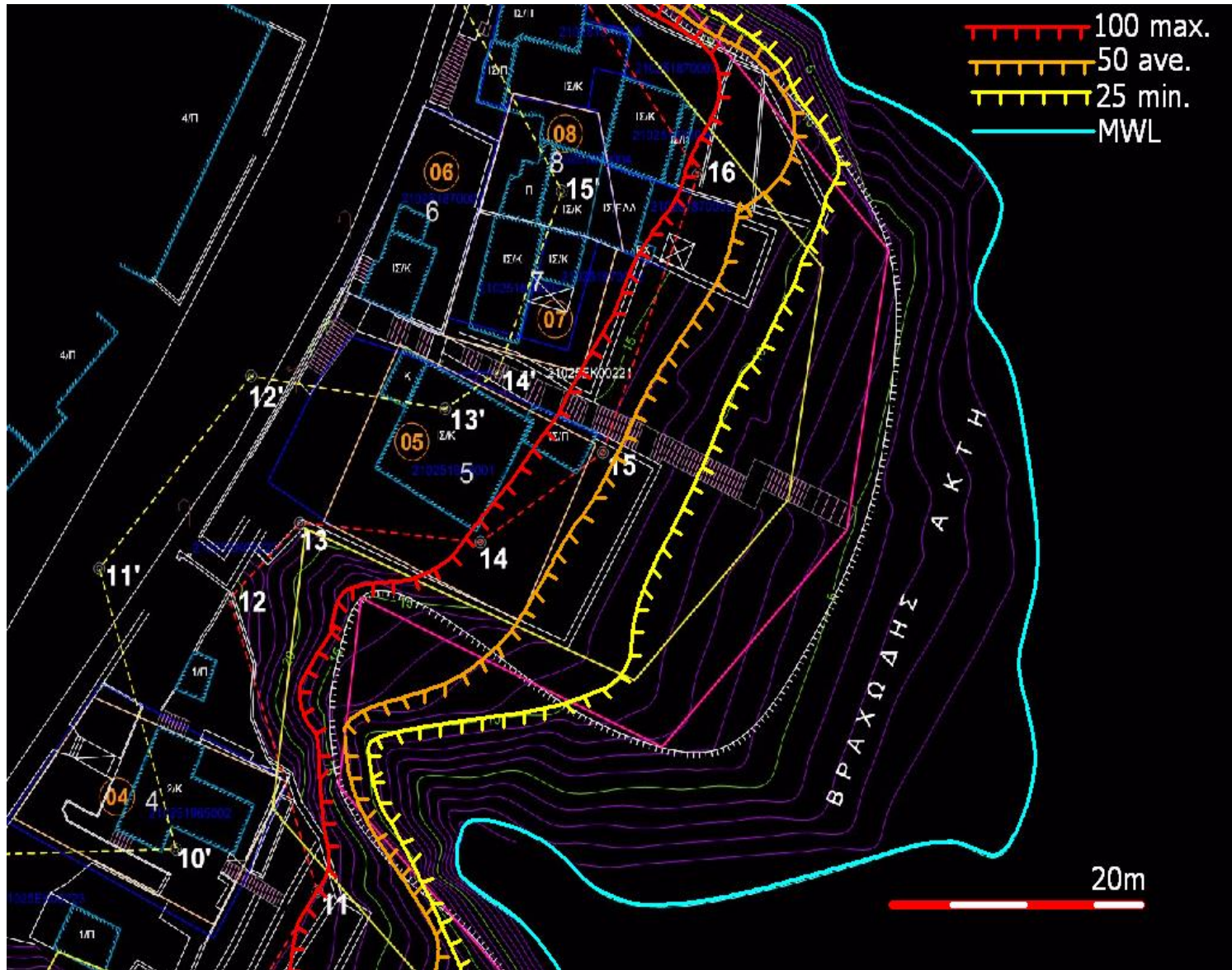
Western part of the Kavala Municipality shoreline with a) the mean sea level (blue line), and the lines of maximum wave run-up, as a) under the 25-years return period (yellow line), b) the 50-years return period (orange line), and c) the 100-years return period (red line)
