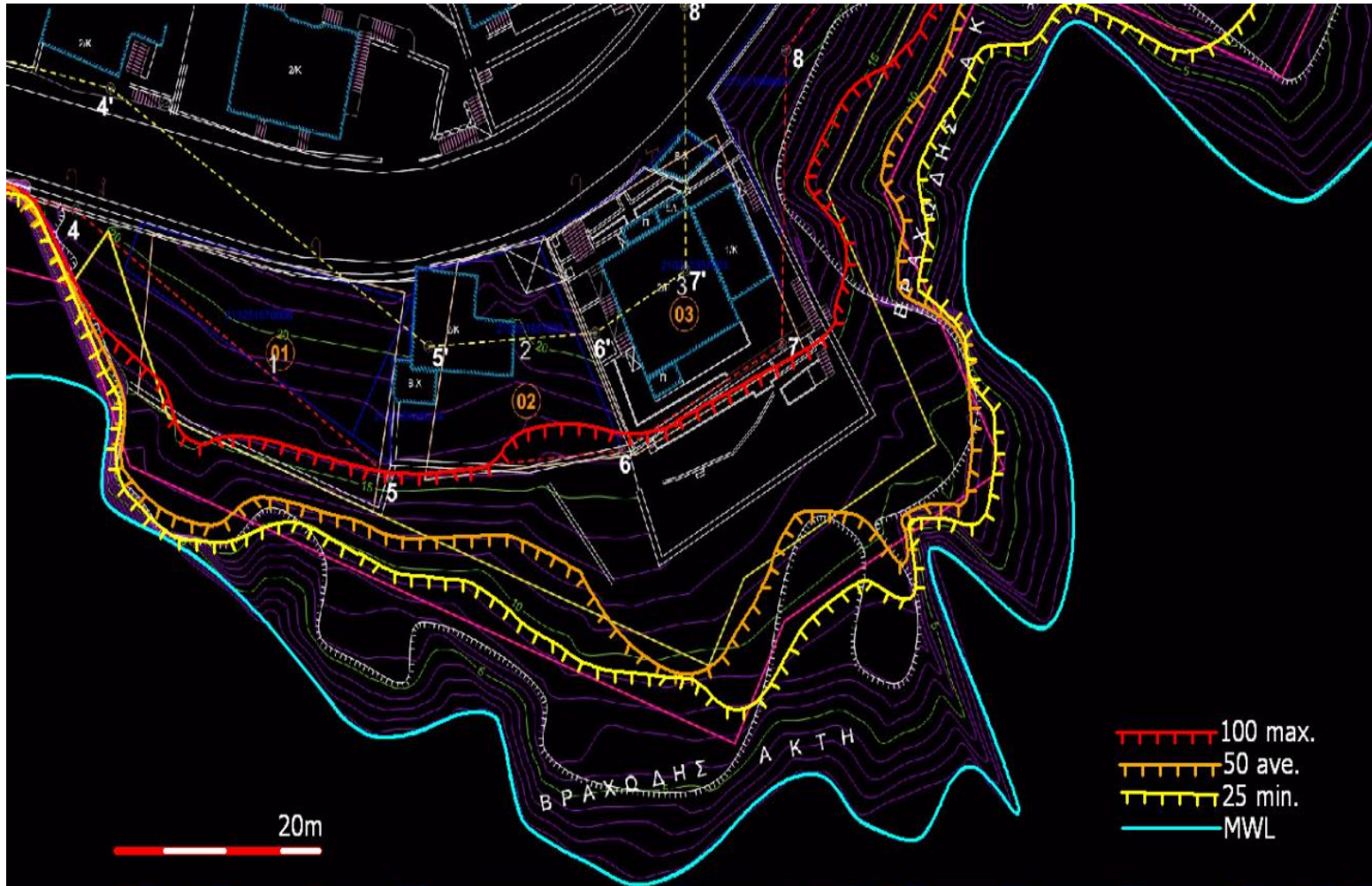
Eastern part of the Kavala Municipality shoreline with a) the mean sea level (blue line), and the lines of maximum wave run-up, as a) under the 25-years return period (yellow line), b) the 50-years return period (orange line), and c) the 100-years return period (red line).
