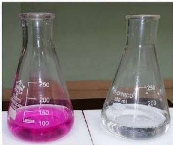
Phenolphthalein end point
