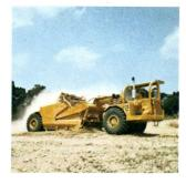
**ELEVATING:** Self-loaded by chain elevators that paddlewheel materials into bowl. Chops and mixes as it loads.
