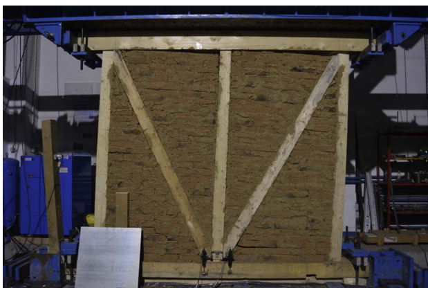
Fig. 44. S2 in the last cycle of the test, at 4.8% shear angle [rad].
