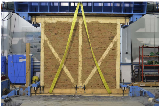
Fig. 29. Position of the wall in the reaction frame.
