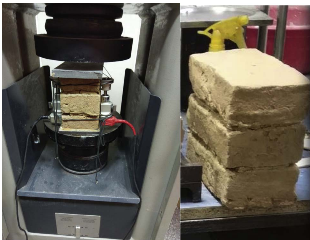
Fig. 30. Layout of specimen and compression test on masonry prisms.
