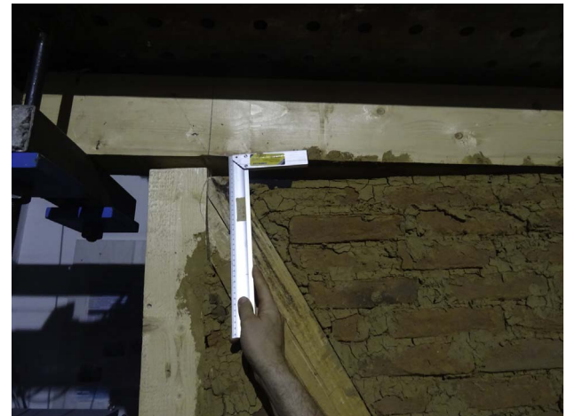
Fig. 45. Upper marginal timber connection significant uplift.
