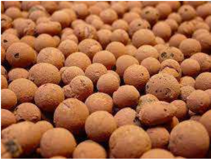
LECA: lightweight expanded clay aggregates
