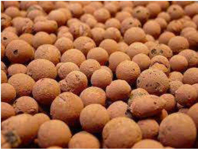
LECA: lightweight expanded clay aggregates
