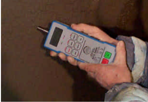
Figure 26: Pocket-sized electronic penetrometer for measuring setting and early age strength development
