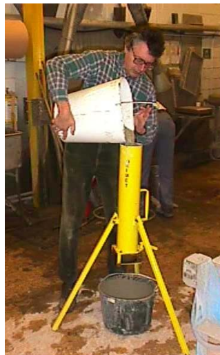
Figure 7 — Filling of the Orimet test
