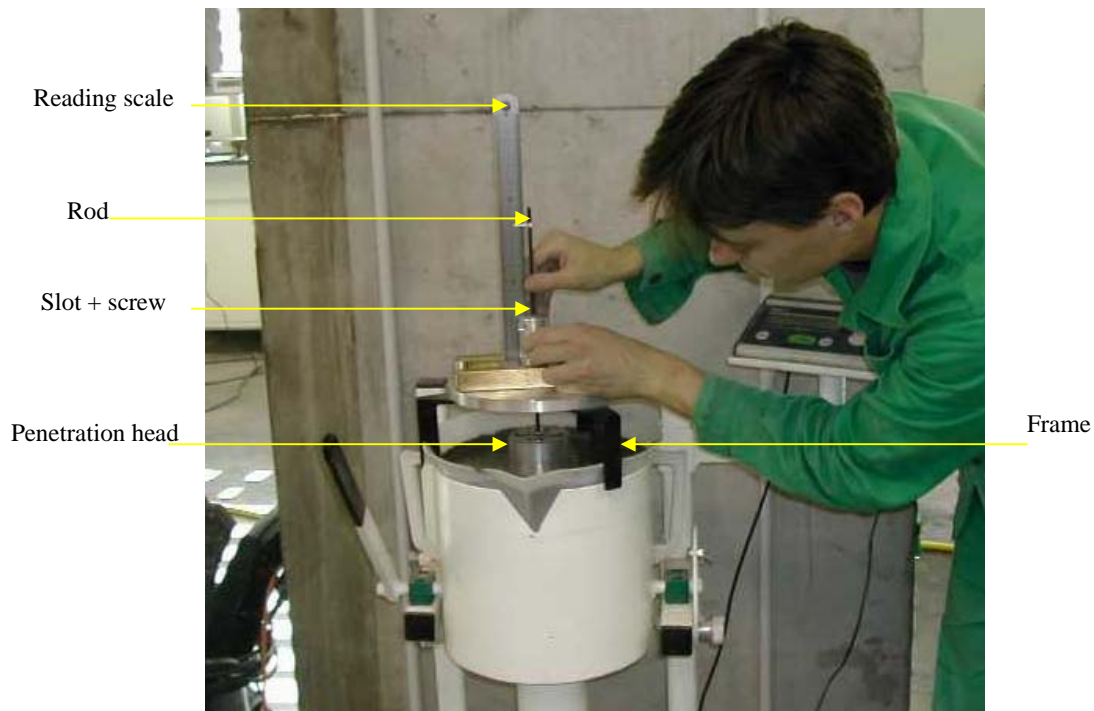
Figure 9 — Illustration of the penetration test
