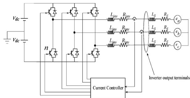
Fig. 1. Current regulated three-phase VSI connected to a back EMF type load (induction motor) through a series impedance.
