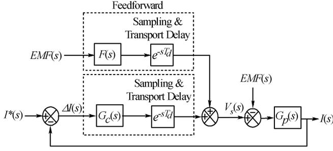
Fig. 8. Average value model block diagram representation of a PI current regulator with delay effects and feed forward compensation.
