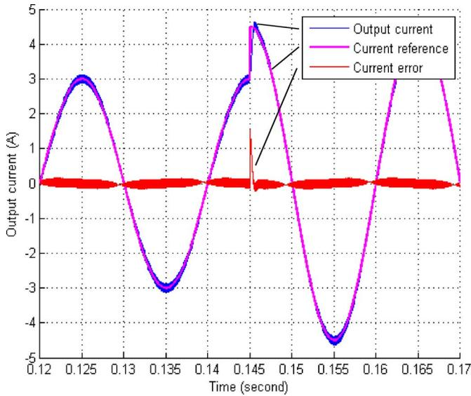
Fig. 3. Simulated response of ideal average value model ac current system with PI regulator,  $k_p = 1$ ,  $\tau_i = 0.0002$ ,  $80 V_{rms}$  back EMF.
