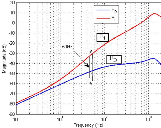
Fig. 7. Tracking and disturbance error for optimized PI stationary frame current regulator  $k_p = 0.58$ ,  $\tau_i = 1.72$  ms.
