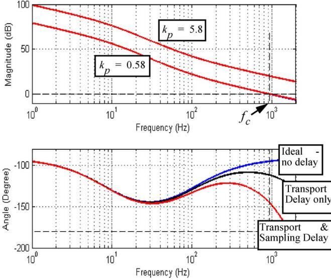
Fig. 6. Magnitude and phase Bode plot of open loop forward path loop gain for ideal controller, transport delay only, transport and sampling delay  $\tau_i = 1.72$  ms.
