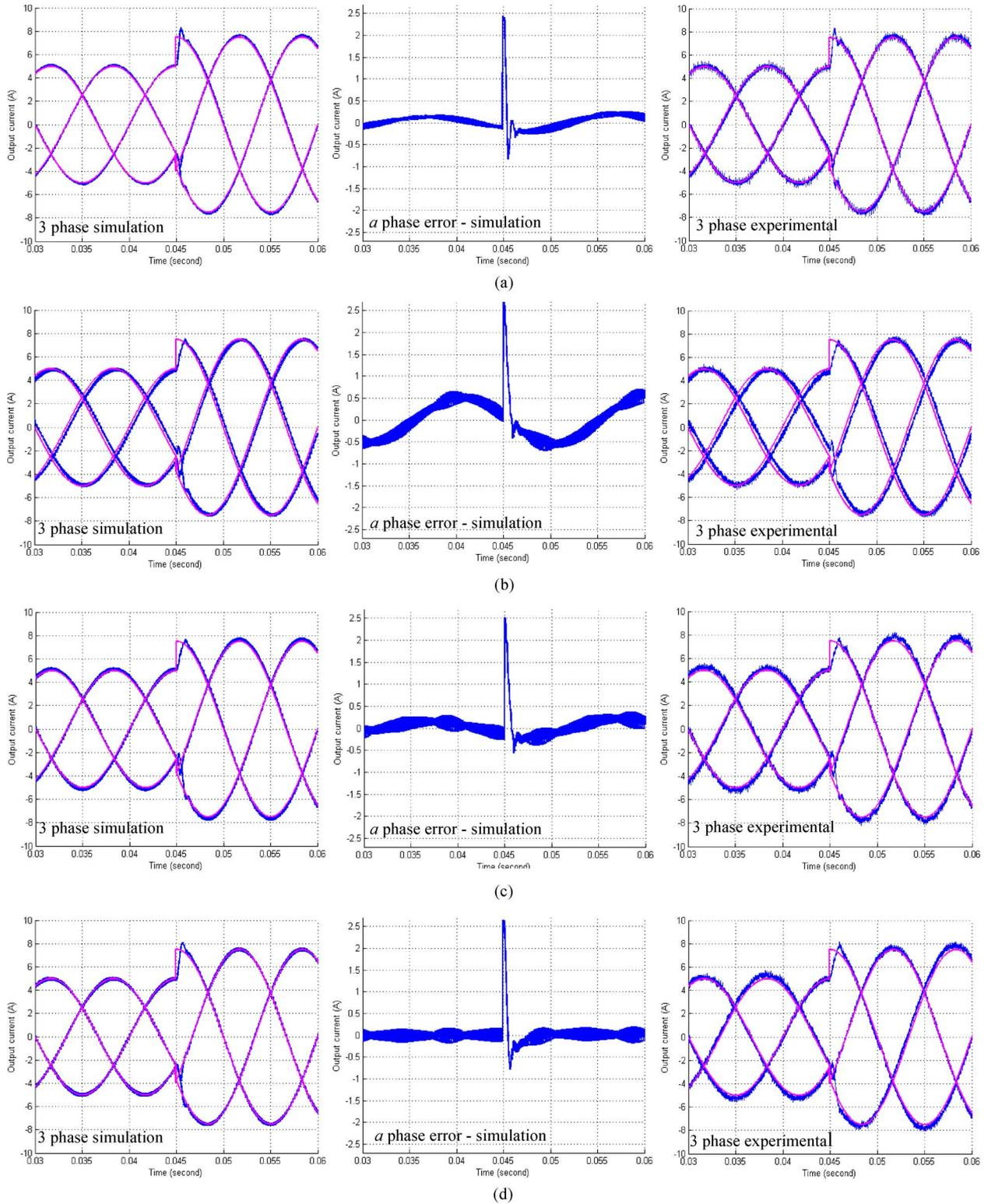
Fig. 10. AC current regulation response of simulated and experimental optimized stationary frame PI and PR current regulators  $k_p = 0.58$ ,  $\tau_i = 1.72$  ms. (a) PI controller, without back EMF. (b) PI controller, with back EMF, no feed forward compensation. (c) PI controller, with back EMF, with feed forward compensation. (d) PR controller, with back EMF.
