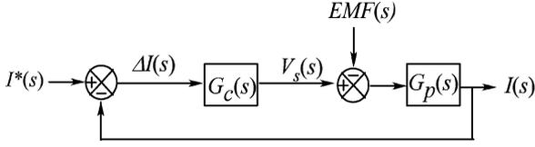
Fig. 2. Average value model block diagram representation of Fig. 1.
