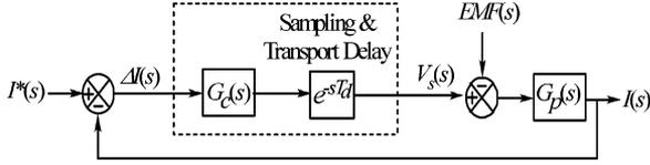
Fig. 5. Average value model block diagram representation of Fig. 1 including the effects of sampling and transport delay.
