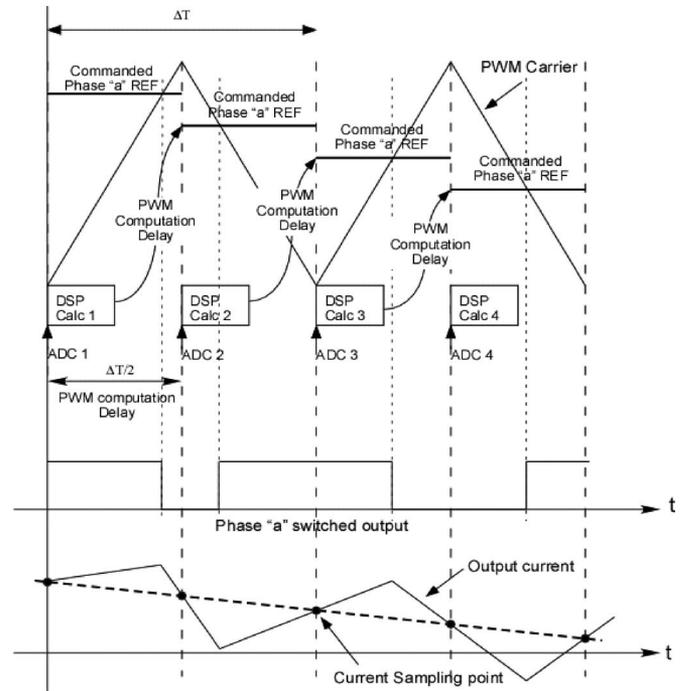
Fig. 4. Transport and sampling delay caused by the PWM process and digital controller sampling/computation.
