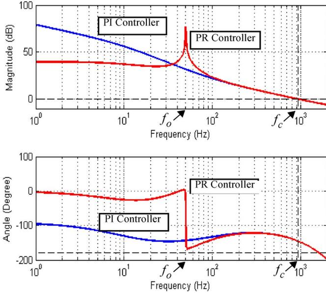
Fig. 9. Magnitude and phase Bode plot of  $G_c(s)G_p(s)$  for PI and PR regulators with sampling/transport delay  $T_d = 0.15$  ms,  $k_p = 0.58$ ,  $\tau_i = 1.72$  ms,  $\omega_r = 0.1$  Hz.
