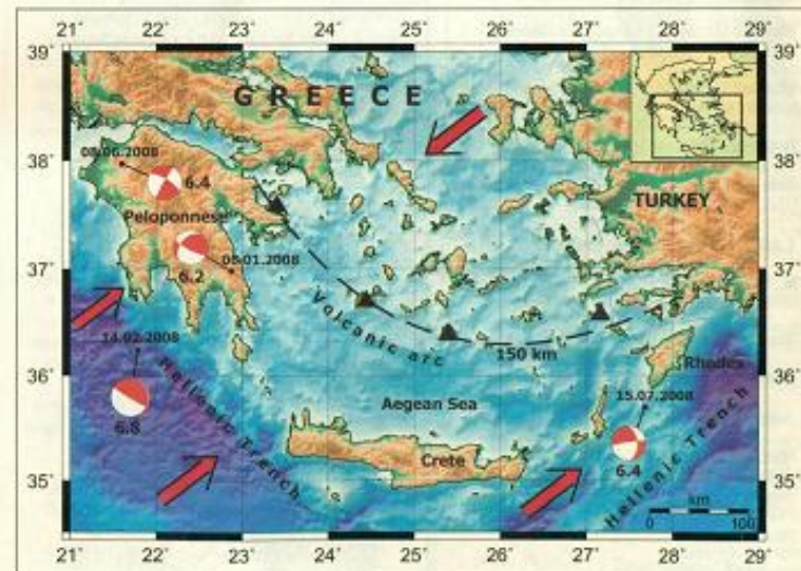
Fig. 1. Seismotectonic elements of the Hellenic Arc and Trench (HA-T) system. Dates, magnitudes, and focal mechanisms (beachball diagrams) of the earthquakes listed in Table 1 are shown (taken from the Harvard earthquake list, http://www.globalcmt.org/CMTsearch.html ). Arrows represent the direction of plate motion, and triangles indicate volcanoes. The dashed line in the volcanic arc indicates the position of the earthquake epicenters at depth of 150 kilometers where magma is generated along the descending Mediterranean lithospheric plate. The box in the inset shows the location of the study area.
