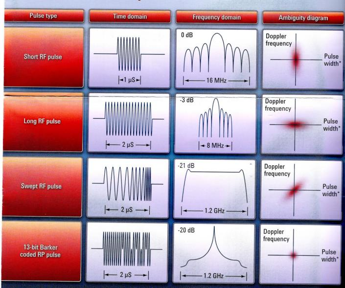
By utilizing pulse compression techniques (modulation), long pulses with lower peak nower can be used without sacrificing range resolution. Processing gain in the receiver compresses the received pulse, which restores the high range resolution of narrower pulses and maximizes the detectable range. The ambiguity diagram illustrates location accuracy (horizontal axis) and Doppler frequency shift tolerance (vertical axis).
