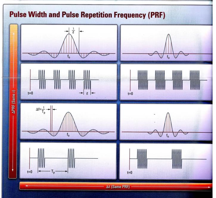
Power, pulse repetition, pulse width, and pulse modulation are traded off to obtain the optimum combination for range and resolution. For simple RF pulses, range resolution varies inversely with pulse width, but narrow pulses drive up peak power requirement Similarly, the maximum unambiguous range varies inversely with PRF. However, pulse modulation radically affects these relationships.
