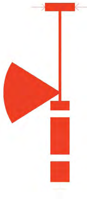
Fig. 5.31 Layout of Bias Network
