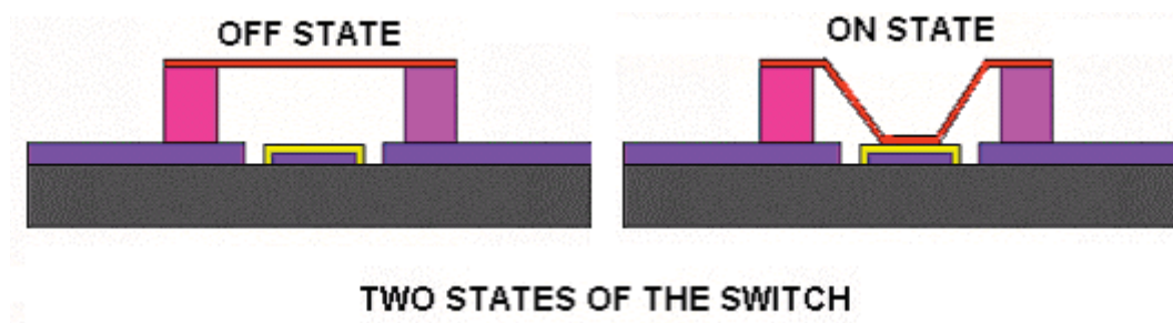
Fig1. Geometry of the RF MEMS Shunt Switch in ON and OFF State
