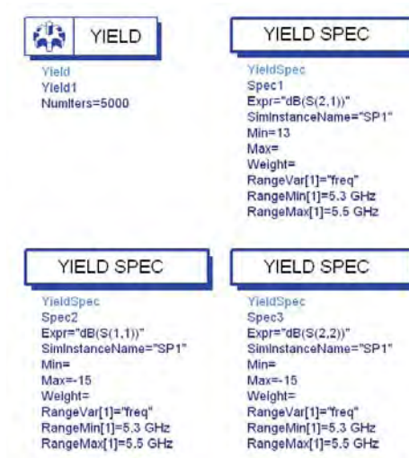
Fig 12. Yield Analysis setup for statistical analysis in simulation
