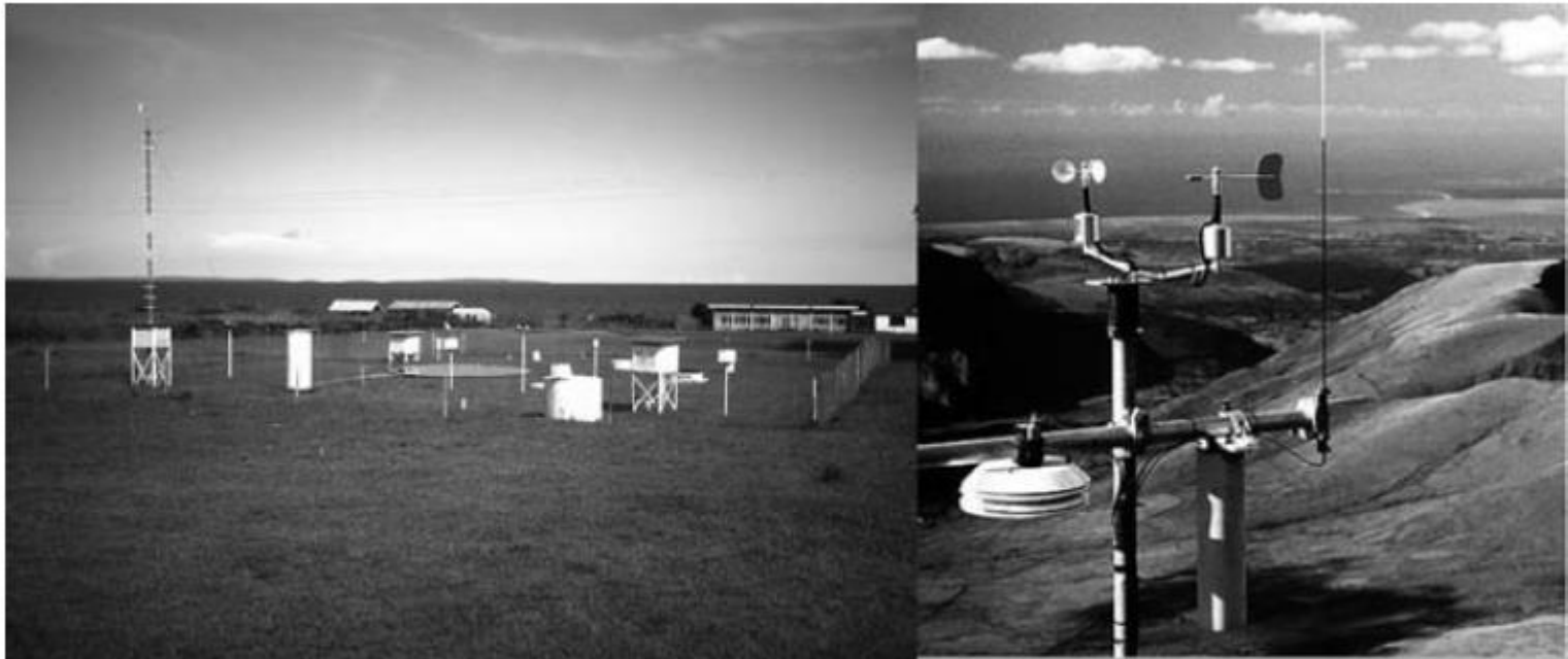
Example of (a) a manually operated weather station and (b) an automatic weather station installed at the top of Mount Snowdon in Wales, including an antenna for radio telemetry of data (© Crown Copyright 2008, the Met Office)
