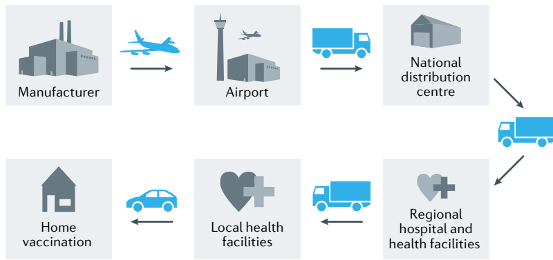
Fig. 3 | The cold chain of vaccines. The cold chain is a temperature-controlled supply chain of the people, equipment and protocols used in the transportation, storage and handling of vaccines from the manufacturer to the patient.
