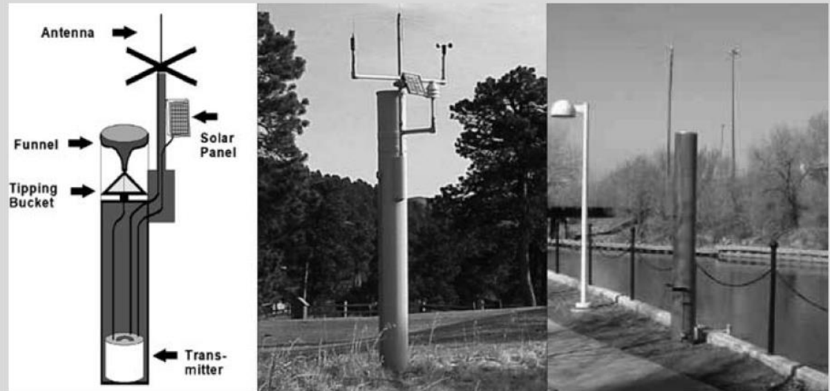
Principles of operation of a radio-reporting rain gauge (NOAA/NWS 2005) and illustration of an ALERT weather station and combined rain gauge and streamflow gauge (Stewart 2009)
