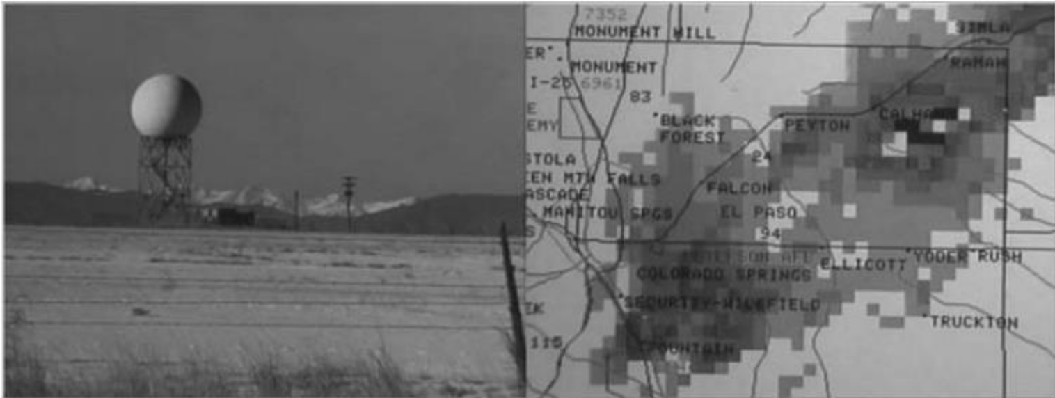
National Weather Service WSR-88D Doppler radar at Pueblo County, Colorado, USA and example of Storm Total Precipitation output ( http://www.crh.noaa.gov/pub/?n=/radar_about.php )
