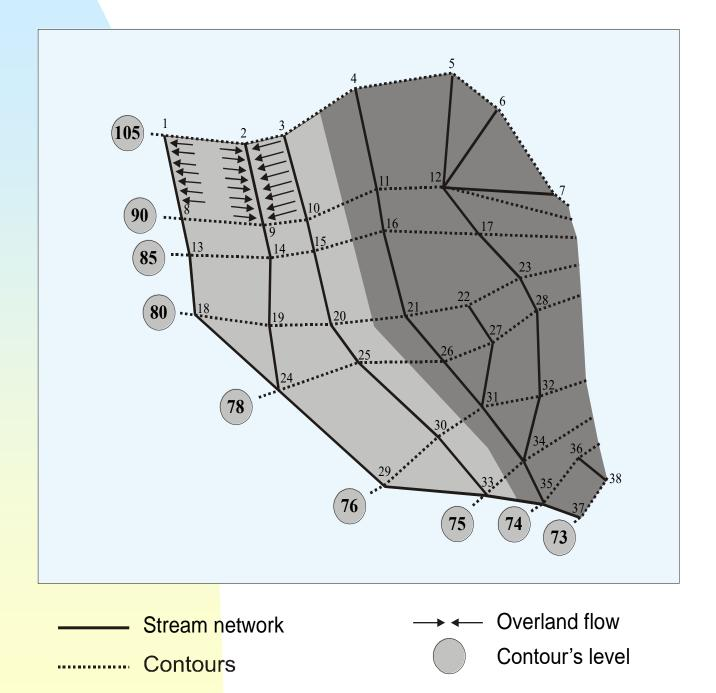
The model substitutes each finite element with a V-shaped overland flow element of equivalent area, which consists of two equal orthogonal planes connected at one side of length L
